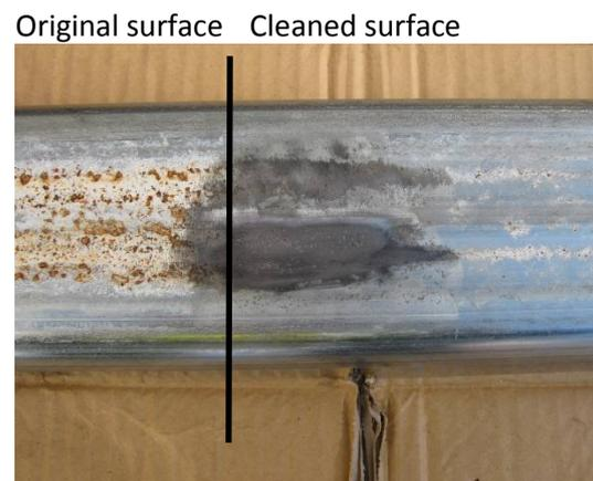
**Picture 3. White rust repair using Wire brush wheel**
